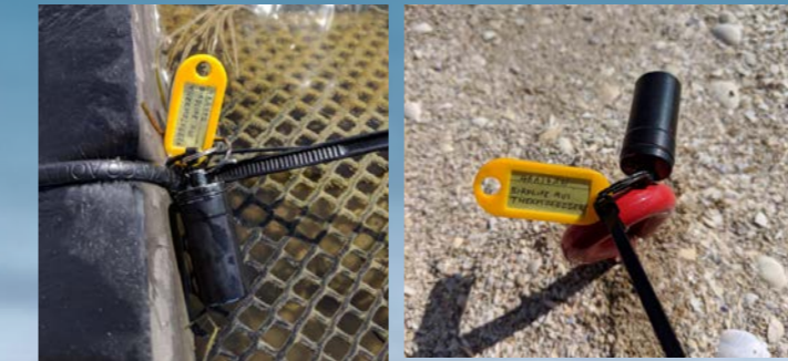
Thermologgers attached to the floating roost (left) and a small screw anchor at a natural roost at Port Philip Bay (right).
